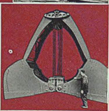
Light-weight construction increases capacity 20%. This gigantic coal bucket built of USS COR-TEN is among the largest ever built. Weighs 17,000 lbs. Will pick up 24,000 lbs. of coal at one bite. Weight-capacity ratio is 1 to 1.4 as compared to 1 to 1 obtained by conventional steel construction. Built by Robins Conveying Belt Company, Passaic, N. J.
