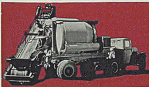
"The Rex modern cone drum of the Rex Moto-Mixer is built of USS MAN-TEN steel of 80,000 lbs. tensile strength for lighter weight, greater strength and longer life. We find that it resists the abrasive action of pounding concrete inside the drum and consequently will prolong the life of the mixer." (Chain Belt Company, Milwaukee, Wis.)
