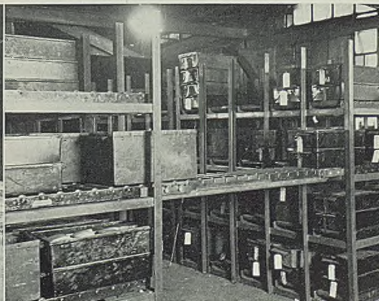
Fig. 18—Crane truck also serves tote box rack equipped with roller conveyor sections
