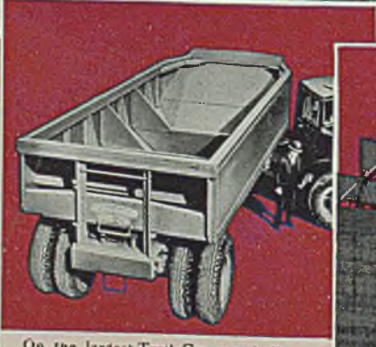
On the largest Trail-Car ever built — 33 cu. yds. capacity. "In designing our Trail-Cars for automotive haulage we were confronted with the necessity for reducing the weight to a minimum, while still using a steel which would resist abrasion. We found these qualities in MAN-TEN Steel, and it has given us entire satisfaction." (The Austin-Western Road Machinery Co., Aurora, Illinois.)
