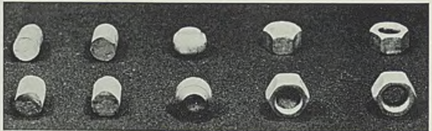
Fig. 7 —The sequence of operations in making a nut in a scrapless nut machine are shown in this illustration. From paper of Roy H. Smith
