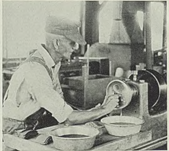
Applying the radial sunray finish on the inside surfaces of hollow ware is a manual process as illustrated here. This operation is known as spinning
