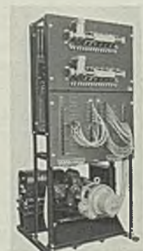
Fig. 2-B—Rear of differential cut-out and plug-in panel assembly
