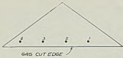
Fig. 4—Rockwell B hardness values of 0.17 C., 1.95 Ni., 1.00 Cu. steel plate after torch cutting and after reheating with torch to anneal:
