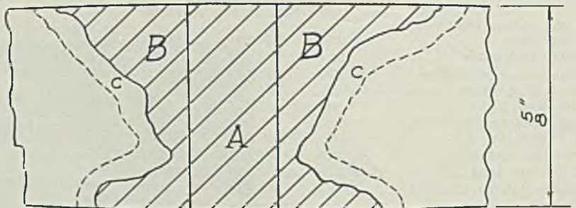
Fig. 2—Analysis of nickel-copper plate and weld using low-carbon electrode with 0.70 per cent molybdenum in the coating:
