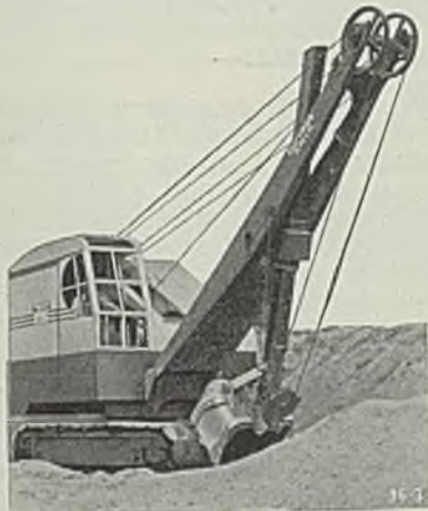
New Bucyrus-Erie \frac{3}{4} -yard excavator weighs 16 tons and has an air conditioned cab
