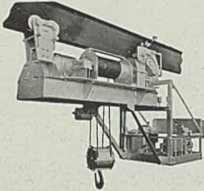
Hydraulic brakes control the movement of this 10-ton Euclid monorail hoist
