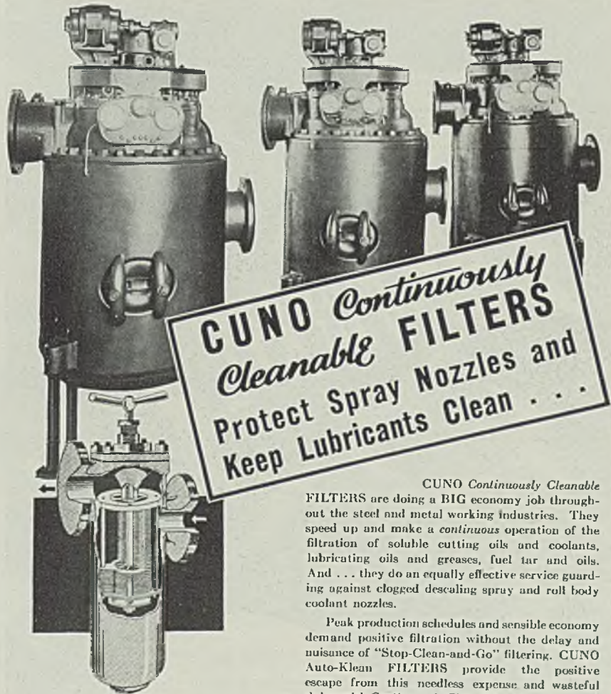
Schematic section of a typical CUNO FILTER, showing direction of flow. Your substance enters the filter case and passes under gravity, pressure or suction head through the closely spaced filtering discs which catch the suspended solids. Then, rotation of the entire element, either manual or mechanical, against the stationary cleaning blades, combs out the filter and drops the unwanted substance to the ample sump below. The filtered and cleaned substance rises through the interior of the cartridges and passes out through the outlet indicated.
