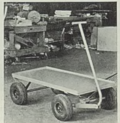
Pneumatic tires are a feature of the electrician's truck built by Saginaw Stamping and Tool Co.
