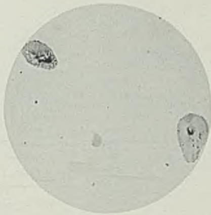
L EFT and center—As cast condition, 19 per cent chromium, 29 per cent nickel, no etchant used. This shows type and dispersion of inclusions. Left 100X, center 500X. Right—Same steel etched in aqua regia glycerine. 100X
