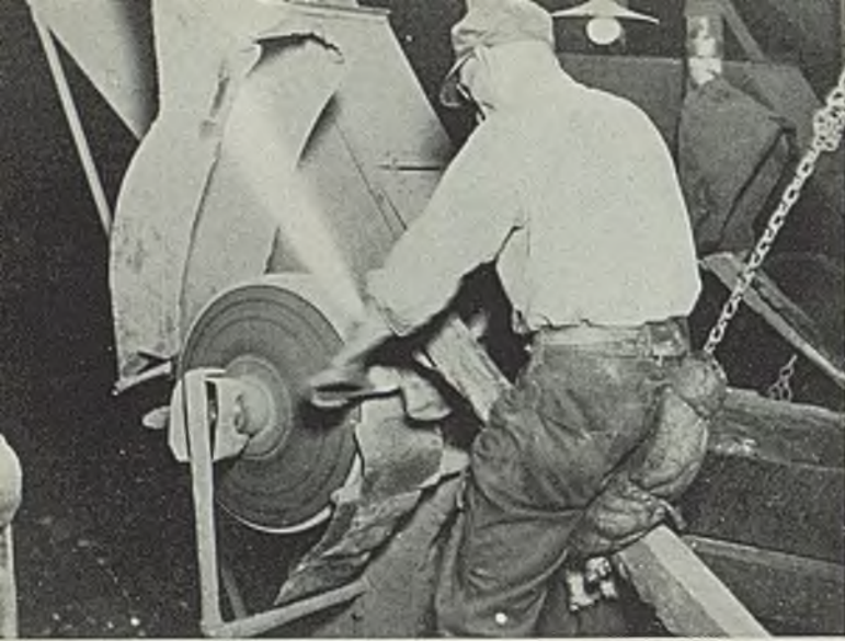
The entire ax surface is ground on a manufactured alumina wheel as illustrated here. The operator keeps the ax in constant motion and exerts the necessary grinding pressure by the weight of his body
