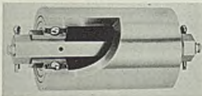
Cut-away view of ball bearing roller showing hexagon axle which prevents rotation of inner ball race
