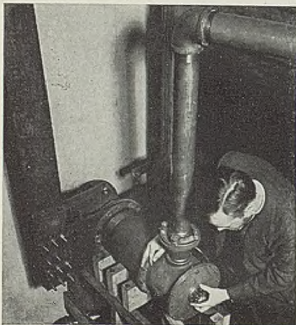
Developed by Dr. Francis Bitter at Massachusetts Institute of Technology, Cambridge, Mass., the magnet produces a permanent magnetic field with an intensity 150,000 times greater than that of the earth. It will be used for fundamental studies of the effects of intense magnetic fields on matter, especially at low temperatures in the neighborhood of absolute zero, which is 469.69 degrees below zero Fahr.
