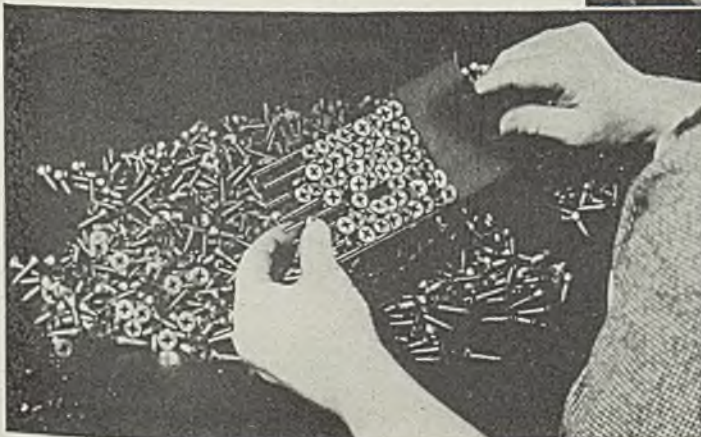
FIG. 1 (right)—Tote boxes containing screws are delivered to the inspector's bench by conveyor. Dumped onto the bench, the screws are inspected as the girl rolls them individually into the opening of the drop delivery chute. They fall into another box which is moved away on a conveyor belt. Fig. 2 (below)—Heads of recessed head screws are minutely inspected as shown here
