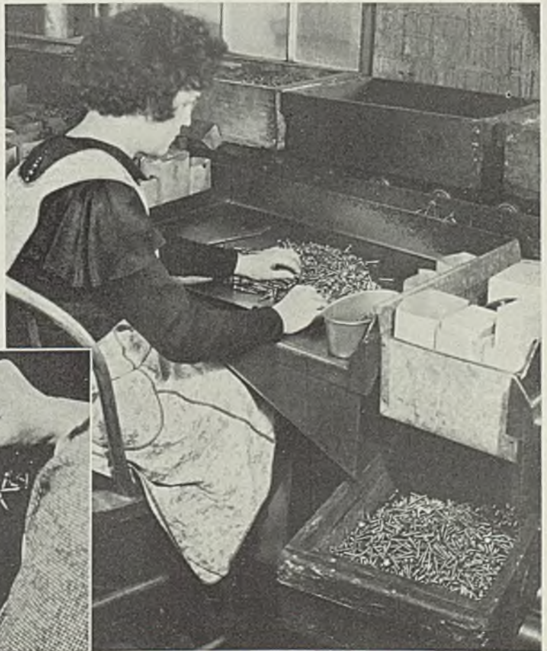
FIG. 1 (right)—Tote boxes containing screws are delivered to the inspector's bench by conveyor. Dumped onto the bench, the screws are inspected as the girl rolls them individually into the opening of the drop delivery chute. They fall into another box which is moved away on a conveyor belt. Fig. 2 (below)—Heads of recessed head screws are minutely inspected as shown here
