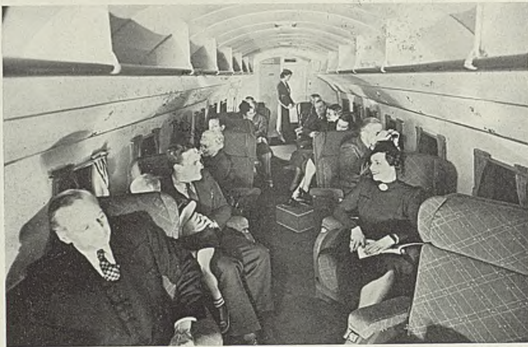
SPACIOUS , unobstructed cabin provides comfortable chairs for 14 passengers, with racks for baggage. Mail and air express is carried in a separate section
