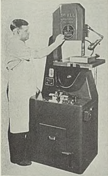
Continent Doall contour saw equipped with the new speed indicating dial
