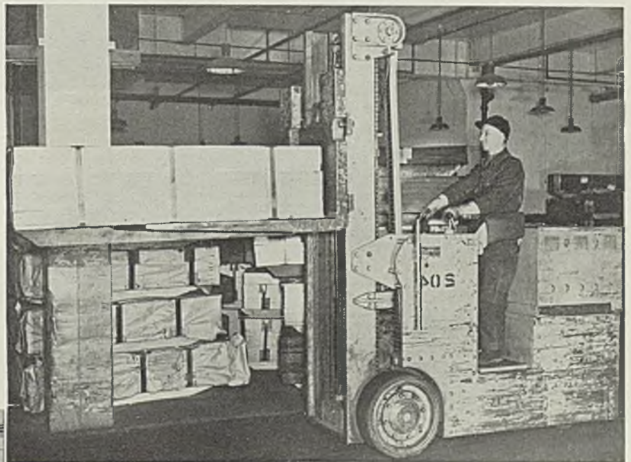
FIG. 1 (right)—A fleet of approximately 150 electric industrial trucks are kept busy in the Buick plant. The fork truck shown here is handling strapped packs of sheet steel
