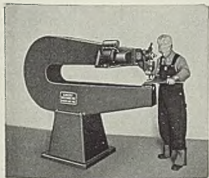
Libert high speed shear designed for use with irregular shapes
