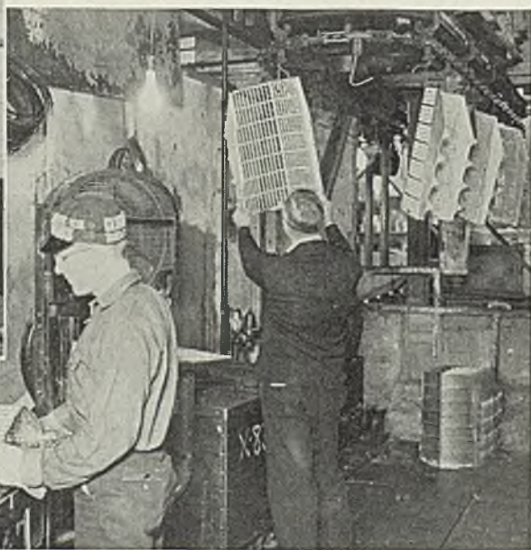
At top left is shown Precision's latest machine for die casting grills at pressure of 3800 pounds per square inch; dies are locked under total pressure of 2400 tons by hydraulically actuated toggle mechanism. At bottom is a close up view of dies in which Olds eight grills are cast. At top right castings, while still hot, are placed over wood form and rough flash broken from them; they are stood on end to cool and then are hung on a chain conveyor and transferred to cleaning department
