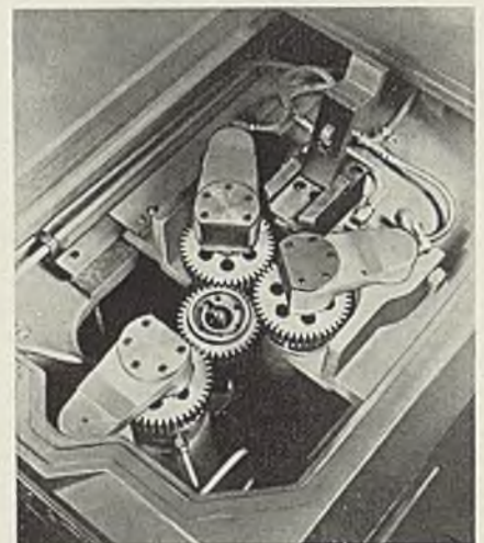
Bolender gear burnishing machine is a product of Cimatool Co., Dayton, O.
