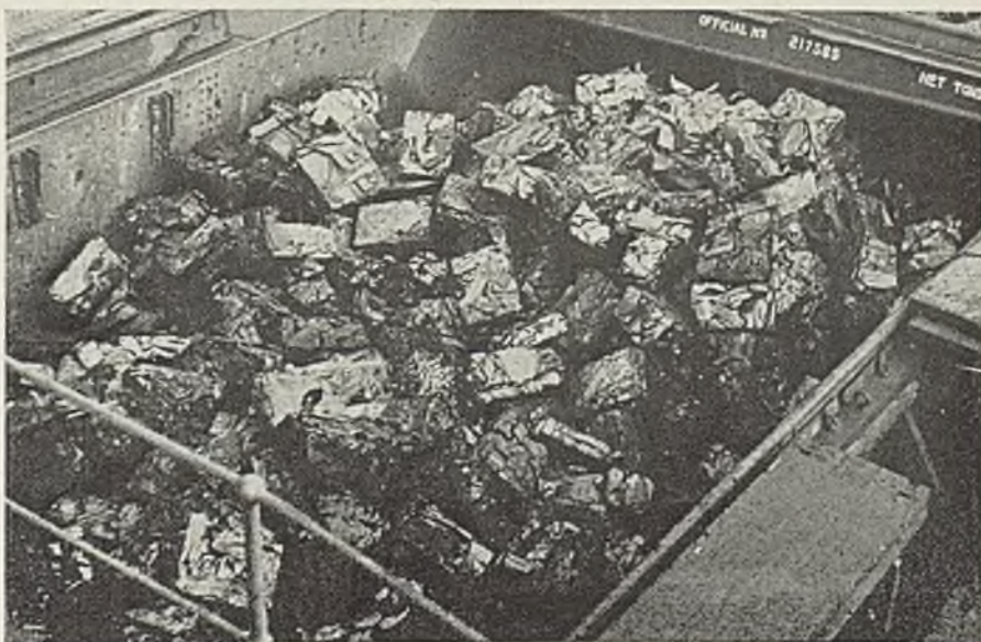
Bundled scrap: Many large metalworking companies now are preparing and shipping their scrap direct to consumers. A larger proportion of scrap is being separated and prepared, according to analysis
