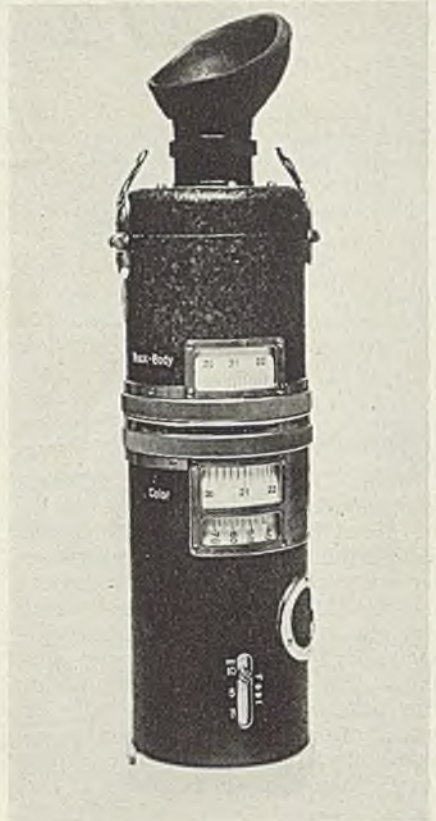
Pyro Bi-Optical pyrometer ascertains both black body and actual temperatures simultaneously
