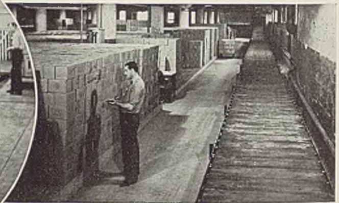
Motors in basement storeroom stacked so that precise inventory may be taken at moment's notice. Wide slat conveyor at right travels length of storeroom and out through tunnel to box cars in which shipments are made. Electric truck and skids are used to bring loads to conveyor
