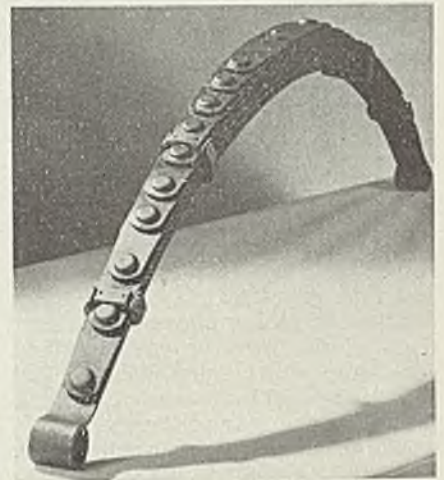
D EPRESSIONS in ends of leaves are formed in the steel to accommodate button inserts
