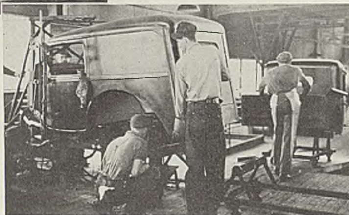
13 —Bantam bodies, above, are electrically welded. Ingenious welding fixtures are used to locate the various sections in place and bring the welding electrodes into position.
