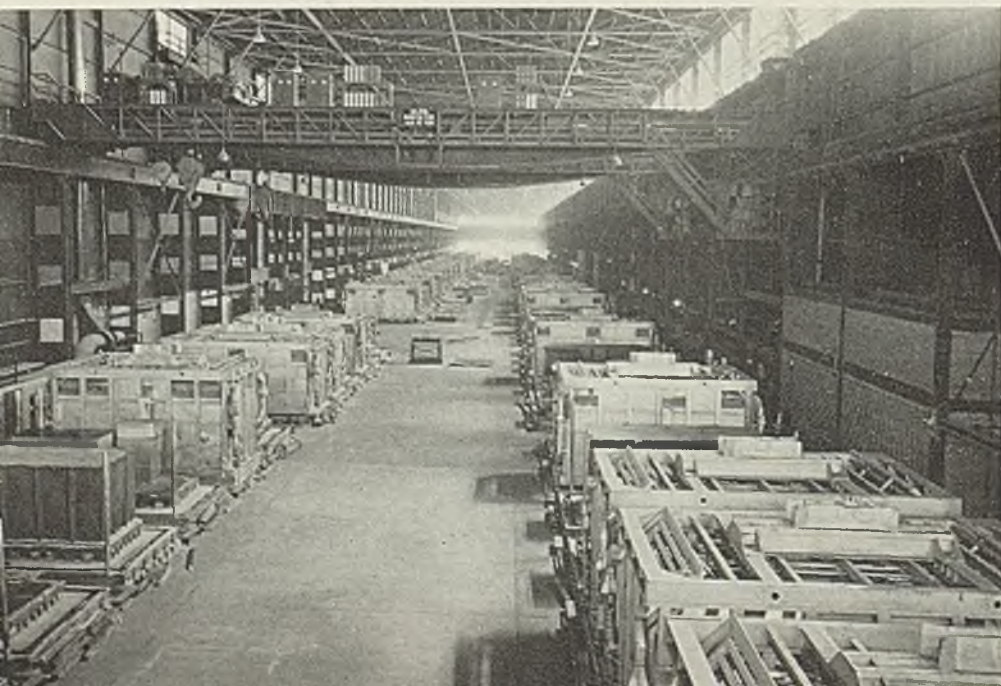
Fig. 1—The box annealing building is about 1000 feet long and 100 feet wide. There are forty-four furnaces arranged along a central aisle
