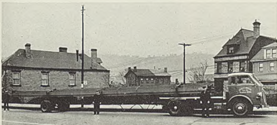
■ Seventeen tons of 60-foot steel members are hauled by this tractor-trailer outfit. Tractor is an Autocar cab-over-engine streamlined model owned by Charles Rosen, Pittsburgh, a contract hauler for a leading steel interest
