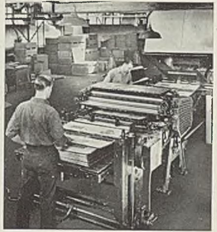
After lithographing, the sheets receive a final coating of clear, alcohol-resistant varnish for protection and a lustrous finish
