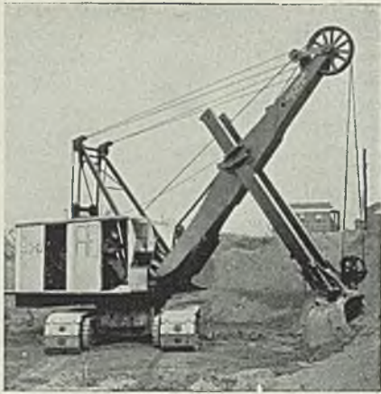
Bucyrus-Erie excavator is easily converted into a shovel, dragline, clamshell or lifting crane
