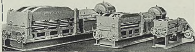
For Production leveling of all material 1/4" to 36 gauge.
