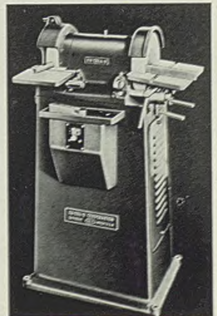
Fig. 1—Left—Ex-Cell-O style No. 46 carbide tool grinder for use with diamond wheels, vitrified cup wheels and lapping disks
