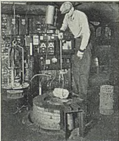
Removing a basket of Carburized Bolts, United Screw & Bolt Co., Cleveland, Ohio
