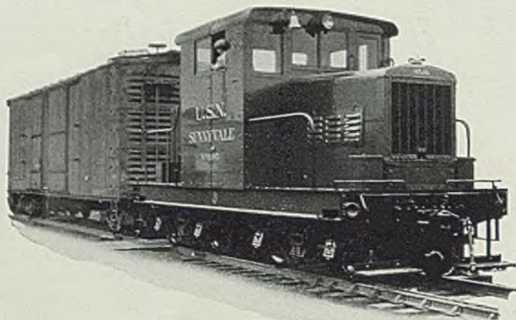
45 Ton Locomotive especially suitable for economical interplant switching service.
