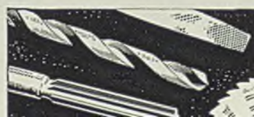
Tool life is greatly increased by chromium plating
