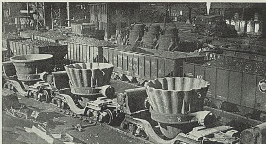
CORRUGATED cinder pots which are not subject to cracks and bulges as a result of severe tem- perature changes
