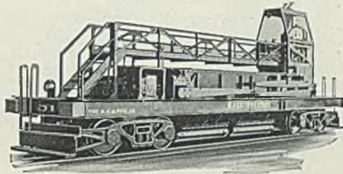
20 Ton — Double Compartment Scale Car. Journals provided with self-aligning anti-friction bearings. Equipped with Atlas Indicator and Recorder.
