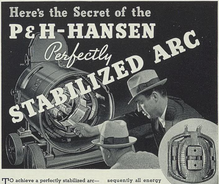
To achieve a perfectly stabilized arc—an arc that "holds" and stays put an arc that "holds" and stays put under all conditions - P&H-Hansen welders embody patented stabilizing coils. These coils are completely imbedded in the main pole flanges—they serve a dual function, as stabilizing and interpole winding. By this unique and exclusive arrangement of the commutating pole windings, P & H-Hansen welders assure the highest degree of arc stability.
