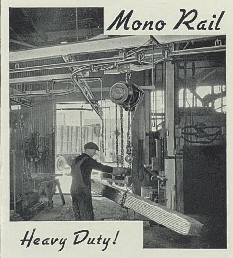
Smooth travel around curves and through switches makes this heavy duty handling of a 3 ton forging billet a simple job on the low-cost, manually operated American MonoRail[System.
