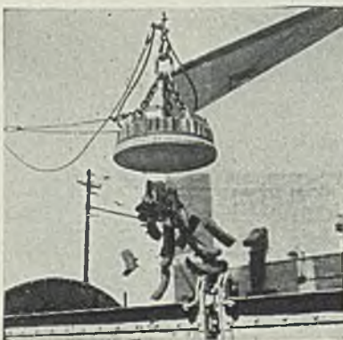
A Non-scattered, Clean Release of Brake Shoes from this EC&M Type SA Magnet is afforded by this Greatly Improved Controller.
