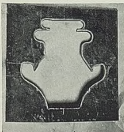
Fig. 3 (left)—Stripper plate for metal cutting die, 18 inches square and \frac{3}{4} -inch thick, flame cut to shape. Fig. 4 (center)—Torch cut gear 7\frac{1}{2} inches in diameter and 3 inches thick. Adjacent is a rough gage for testing contour of the gear. Fig. 5 (right)—Examples of parts flame cut from 6-inch stock for exhibition
