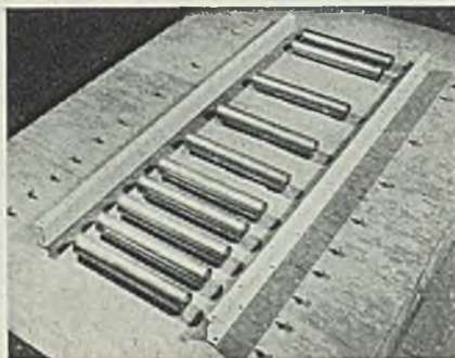
Eastern roller conveyor showing knock down construction
