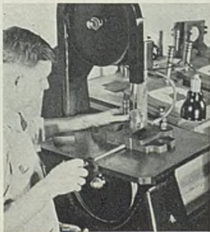
Fig. 7—Cutting out holes in die shoes is an operation which is performed easily on the machine
