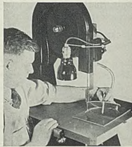
Fig. 8—True circles are made by pivoting the work between centers and revolving it into the saw
