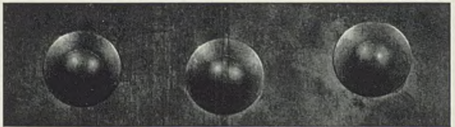
Erichsen or cupping test in thin-gage copper-silicon-manganese sheet, center impression being directly across line of weld
