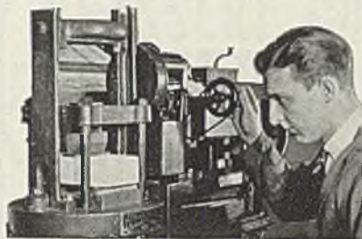
Control Laboratory tests, such as this one for breaking strength, assure uniformly high quality and dependable performance by Armstrong's Insulating Fire Brick in your plant or high temperature equipment.
