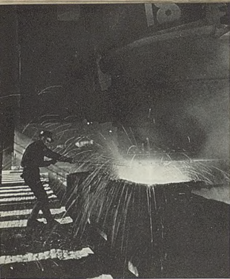
■ As steel is poured into ingot molds, a workman takes a laboratory sample to be used in checking the correctness of analysis. Photo courtesy Carnegie-Illinois Steel Corp.
