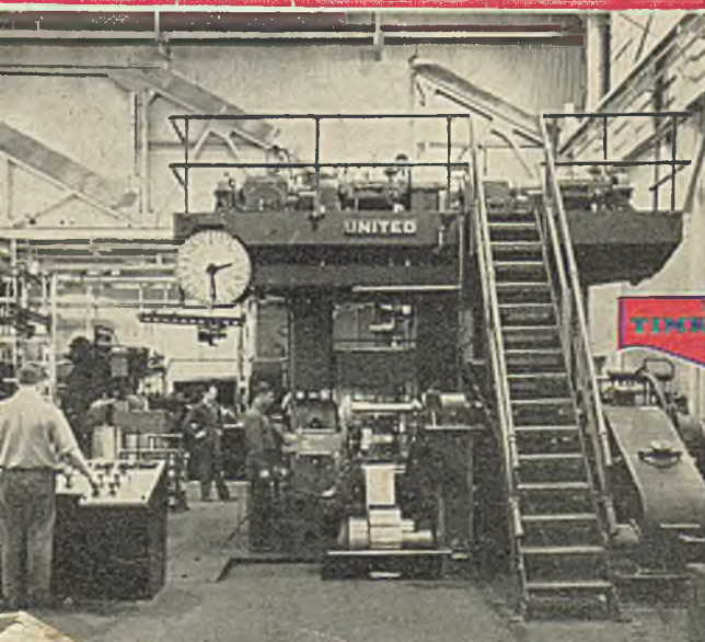
28" United 4-high Reversing Cold Mill equipped with TIMKEN Bearings.
