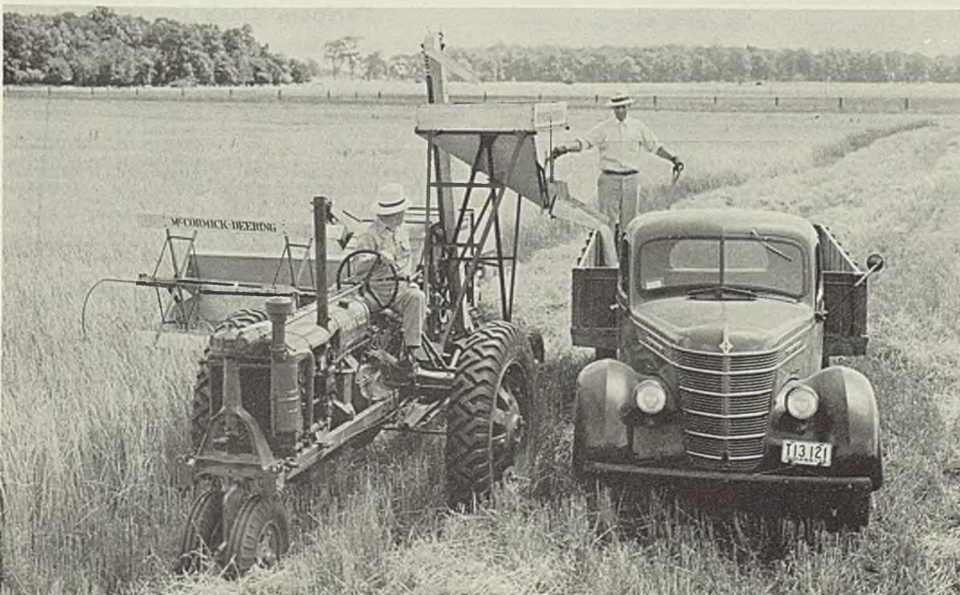
■ Small combine at work with the tractor in harvesting wheat. Threshed grain is seen flowing from the grain tank into the box of the motor truck
