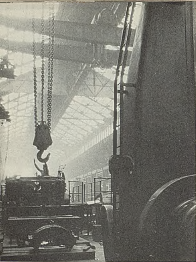
■ For moving heavy loads, an overhead crane gives access to every spot on the shop floor. With suitable slings, loads of about any type or shape can be handled. Photo courtesy Westinghouse Electric & Mfg. Co.
