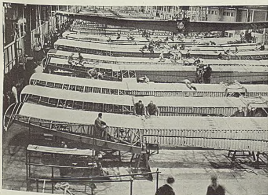
■ View in wing assembly section of a factory "somewhere in England," where Whitley bombers are under construction. These war planes have a range of 1900 miles with a top speed of 240 miles per hour. They are equipped with two engines developing 2000 horsepower. NEA photo
