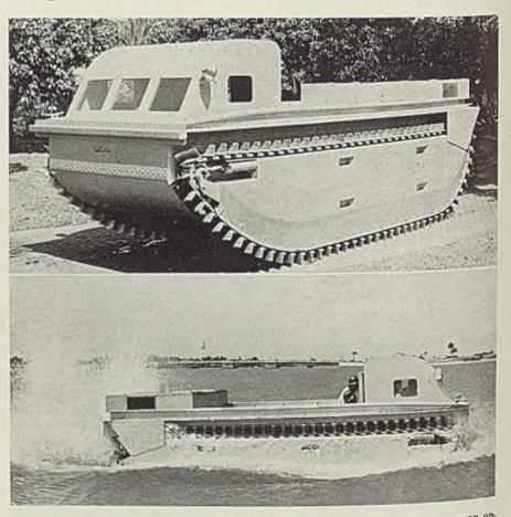
■ In the 1940 model Alligator amphibian tractor built by Donald Roebling, Clearwater, Fla., for work in flooded areas, both land and water propulsion are obtained from an endless chain on either side fitted with curved cleats 6 inches high. On land, top speed is 25 miles per hour; in water, 8.6 miles per hour. Tractor draws less than 3 feet of water without cargo. Hull, 20 feet long, is duralumin, Alcoa 17 ST and has bottom plate of Alcoa 24 ST. Motor
