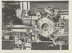
This part is made from chrome molybdenum steel bar stock on a No. 5 Jones & Lamson Ram Type Universal Turret Lathe. All tools and tool holders are standard Jones & Lamson Turret Lathe Tools. A taper turning and boring attachment on the hexagon turret finish bores the taper, straight and radial interior diameters, guided by a former attached to a bar mounted on the headstock. This bar can be swung out of the way when not in use.
