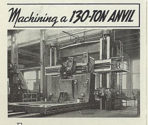
Lirie Foundry Company is operating what is believed to be the largest planer in the United States... The machine takes work 16 ft. 6 inches between the housings by 14 ft. 3 inches under the rail. This planer enables Erie to effect economies in the machining of parts for large Erie steam drop hammers... and to offer its unusual facilities to designers heretofore hampered by existing
