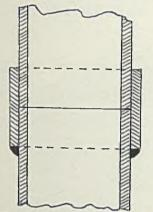
Fig. 4—Slip joint. Lower side of coupling is welded by pipe manufacturer
