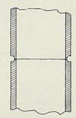
Fig. 6-U-bevel butt joint
