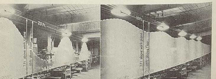
ly alike, the brightness ratio be-tween highly illuminated work and the darker surroundings in general should not exceed ten to one. While measurement by a light meter in footcandles is not an actual determination of brightness, it suffices in most cases for this matter of satisfactory contrast. Hence the common statement that, using gen-
