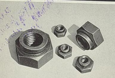
The new Stay-On Lock Nut keeps assemblies tight which are subject to severe vibration. Slotted crown section, eliptical in shape after heat treatment, grips bolt thread like a vise. One-piece design. Can be used repeatedly.
