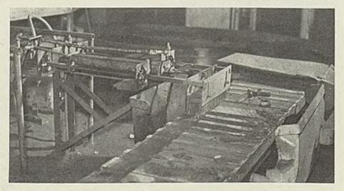
M Automatic broom designed by Buick engineers to sweep sand from mold conveyor line in foundry. Referred to in STEEL, Jan. 15, p. 36, the handle is mounted in an air cylinder arranged to reciprocate the width of the conveyor. Side bars move in rollers and support the broom rigidly
