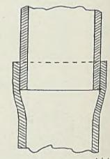
Fig. 3-Bell-and-spigot joint
