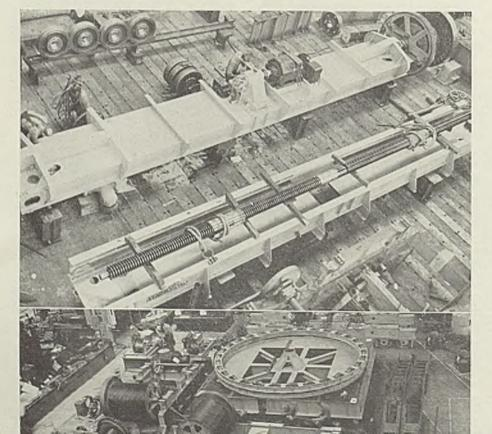
grooved for %-inch wire rope lead lines, the load block being reeved for four parts of line. Mechanism is motor driven through a double set of spur reduction gears to give a rope speed of 78 feet per minute.
