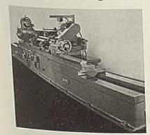
ing work table, fixed grinding wheel unit and a sensitive reversing mechanism which permits grinding up to shoulder of shaft. Traveling work table running on inverted V-ways is superimposed on front bed. Once set, traverse and reversal of traveling work table are automatic and require no further attention.
