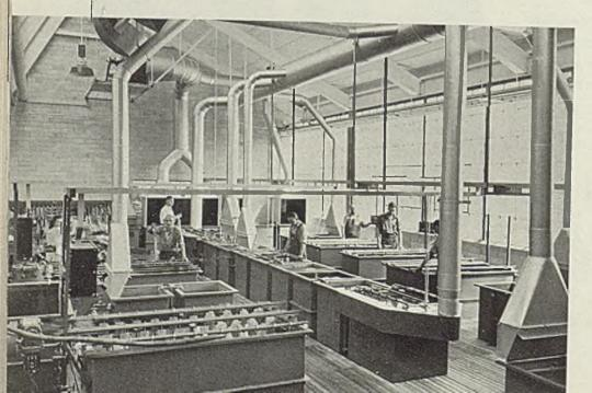
extreme care to assure maxim efficiency in all types of elec plating finishes. In any case, work traverses the minimum tance, is not subject to usel backtracking, nor does work in a one line interfere with other ope tions.
