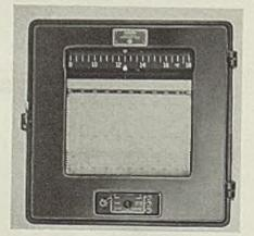
vanometer pointer of less than 0.0001-inch without lost motion. By positioning a friction roller, cam positively determines movement of integral slide-wire contact, recording and control actuating carriage. Integral recording and control mechanism co-ordinates measuring, recording and controlling operations. Slide-wire contact, recording pen and cam follower actuating control cam are assembled as a unit on same rigid carriage. Guaranteed accuracy is ¼ of 1 per cent of scale range.
