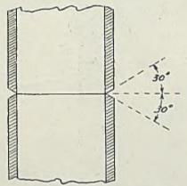
Fig. 1—Symmetrical vee butt joint
