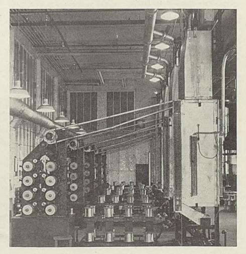
quires the sintering of parts made of pressed, powdered metals at elevated temperatures in a controlled atmosphere. A new mesh-belt conveyor-type electric furnace has been produced for such work. Suitable for operating temperatures up to 2100 degrees Fahr., the heating chamber is equipped with heavy nickel-chromium rolled-ribbon resistors.
