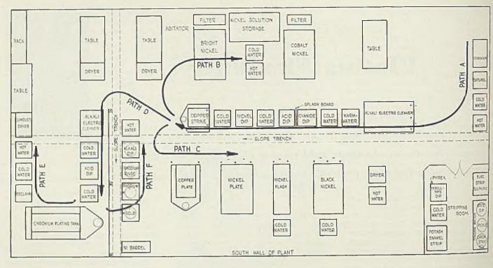
Fig. 3—Layout of general plating section showing the various paths work may follow in receiving the many different finishes and combinations of finishes which can be produced here
