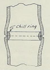
Fig. 2-Double bell joint with chill ring
