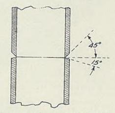
Fig. 5—Asymmetrical vee butt joint
