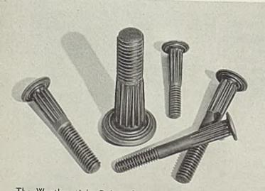
The Weather-tight Bolt is for wood construction. Head of this bolt sets flush with surfoce of wood without counter-boring. Prevents moisture seepage beneath head and from nut end as well. Tapered splined shanks prevent turning when nut is applied.
