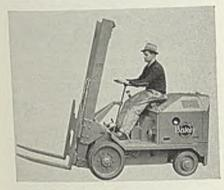
cylinder Hercules industrial gasoline engines designed for continuous operation at high power output and rubber mounted to reduce vibration. Heavy-duty industrial-type transmission and clutch are used, gearbox providing two speeds forward and two reverse. Hydraulic brakes on drive wheels and all controls of automotive type are provided.
