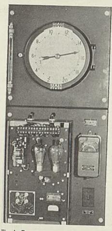
Fig. 1—Temperature control instrument, time clock, control switch and Reactrol control panel without cover at lower left, for gas carburizing furnace
