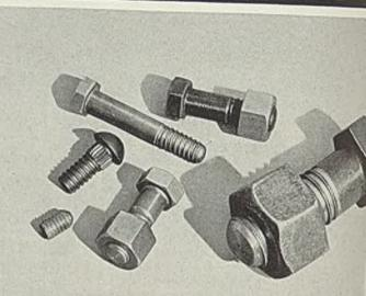
Dardelet Self-Locking Screw Threads may be applied to any type of bolt. Dardelet bolts are unaffected by vibration, loss of initial bolt tension or wear. They have higher tensile and impact strength, and greater endurance limit than standard threads.
