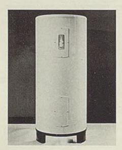
top, is finished in white Calgloss. The rounded edges of top fit smoothly over the body, and front panels are absolutely smooth without cracks or crevices to catch dust and dirt. This heater is available in 30, 40 and 50-gallon sizes with Monel or galvanized tanks, single or twin unit type. Heating is by Calrod hairpin unit and Thermosnap assures utmost economy and automatic operation.
