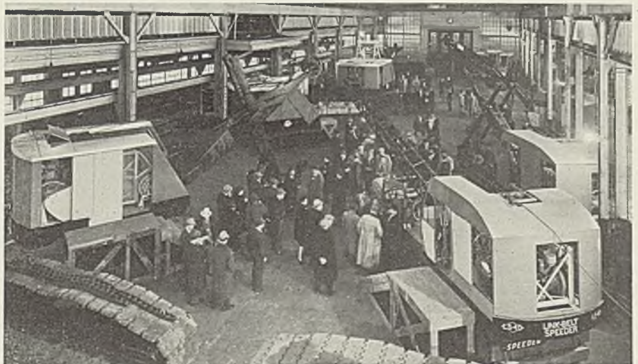
■ Typical of displays at the annual roadbuilders show last week in Chicago, this bay of Link-Belt Speeder Corp., 301 West Pershing road, Chicago, featured a model 570 shovel with a 2½-yard dipper
