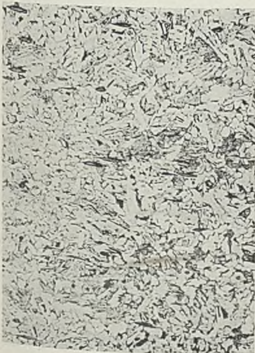
Fig. 6—Micrograph of core of annealed specimen of high-sulphur steel. Manganese sulphide inclusions are clearly visible
