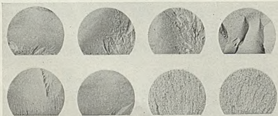
Fig. 1—Fractures of hardened specimens. Hardening temperatures in degrees Fahr., left to right, top row: 1450, 1500, 1550, 1600; bottom row: 1650, 1700, 1750, 1800. Actual size
