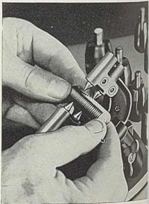
Above: Limit snap thread gages check the pitch diameter of every "Acorn" Die test plug — 100% inspection.
