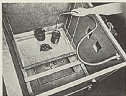
Fig. 2—Larger unit has motor-driven flusher unit shown here. Holds 10 gallons of solvent, will degrease twelve 150-pound loads per hour, has operating area 36 x 30 x 22 inches. These units are made by Phillips Mfg. Co., 340 West Huron street, Chicago
