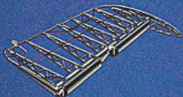
This light, strong rudder frame for a seaplane was fabricated from durable stainless steel by high-speed spot-welding.
