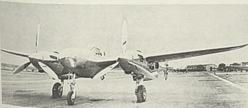
■ Claimed the "world's fastest", this twin-motored Lockheed P-38 interceptor pursuit plane is the first of 70 which will be delivered to United States army air corps. Official photograph by United States army air corps shows ultra-streamlining which makes possible a top speed of around 500 miles per hour. Acme photo
