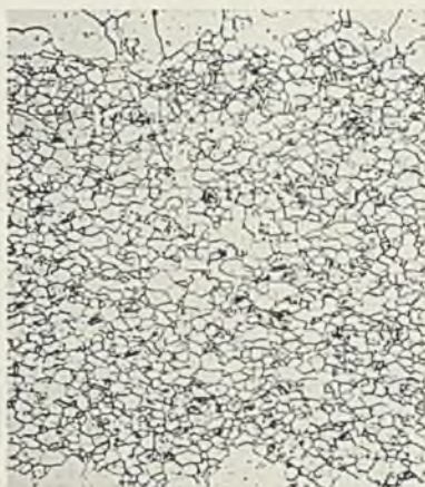
Fig. 15—Elongated 7.5 per cent, annealed at 1200 degrees
