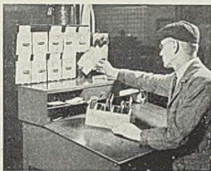
Fig. 2—A foreman can tell at a glance which job is in progress on any machine in his department. Each machine has a portion of the wire rack. When a job is assigned, the foreman simply puts the routing card for that job in proper place in rack
