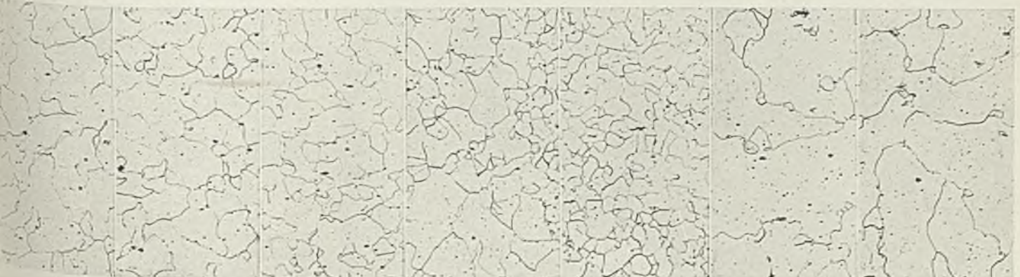
Fig. 23—Elongation increased to 15 per cent, same anneal. Fig. 24—Elongation 20 per cent. Fig. 25—Elongated 25 per cent. Fig. 26—At 1600 degrees, elongation 15 per cent. Fig. 27—At 1700 degrees, elongation 10 per cent. Figs. 28 and 29 were both at 1400 degrees, 5 per cent elongation, but Fig. 28 annealed 2 minutes, Fig. 29 annealed 10 minutes
