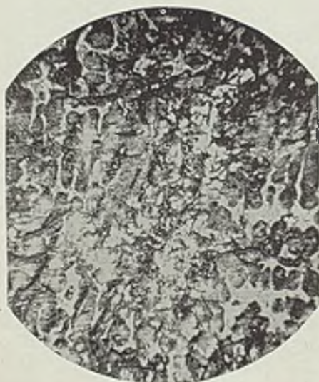
Fig. 1—This material enameled well. In "as cast" condition etched, 200 diameters magnification
