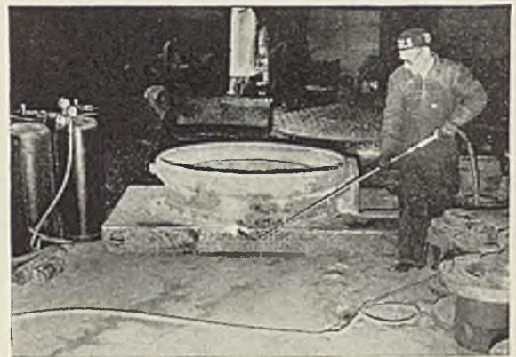
Flame-descaling a large casting with round tip mounted on extension.
