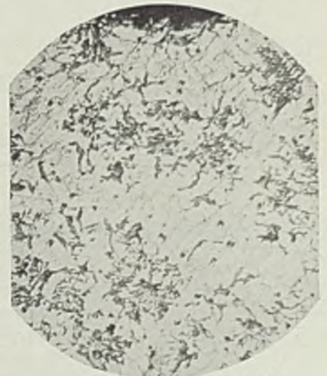
Fig. 8—Section of chilled door lug. Note soundness and graphite distribution. Enameled well. At 200 diameters
