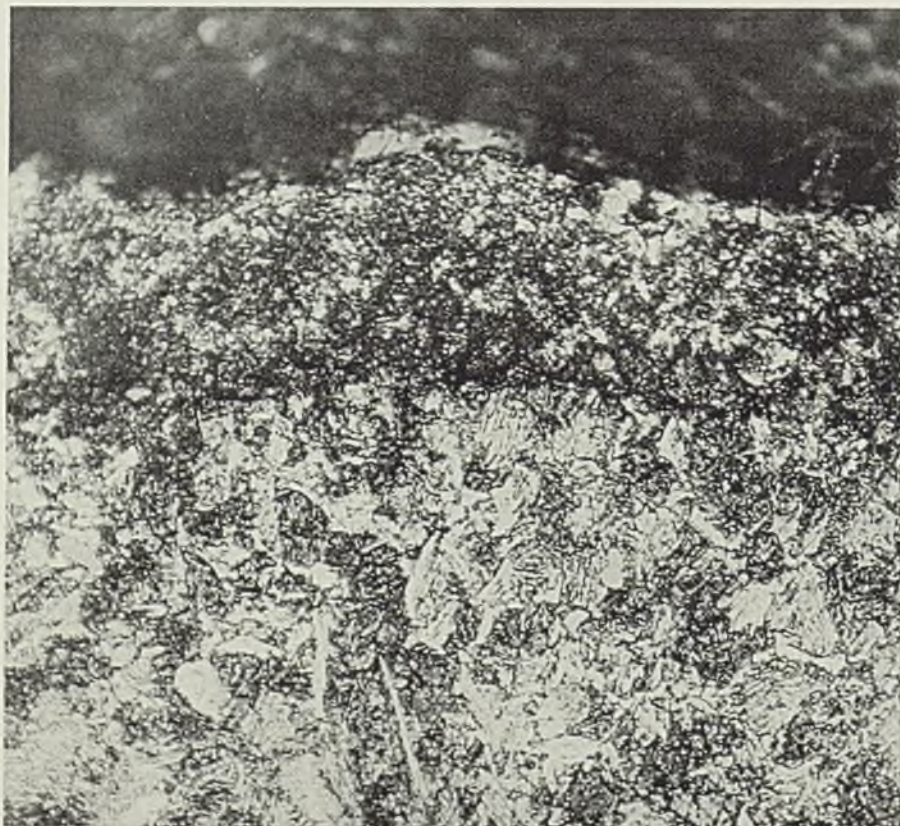
Fig. 7—Properly heat treated malleable iron showing no decarburization at edge. At 500 diameters
