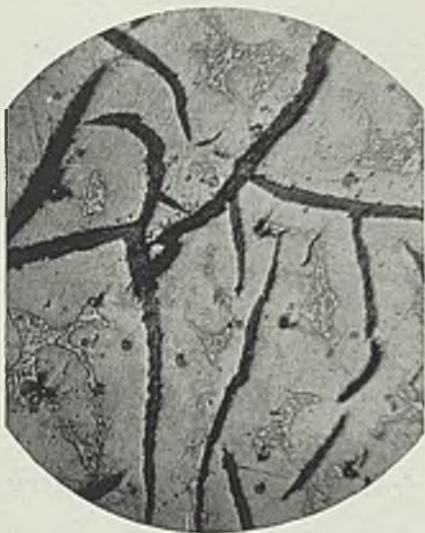
Fig. 4—Coarse graphite distribution. Casting blistered on enameling, magnified 200 diameters
