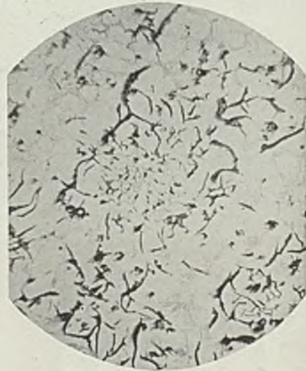
Fig. 3—Graphite of satisfactory fineness as evidenced by good enameling properties. Unetched, 200 diameters
