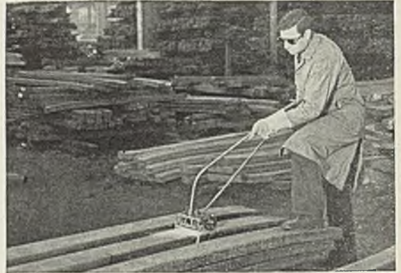
Flame-descaling billets with flat-tip assembly mounted on carriage.
