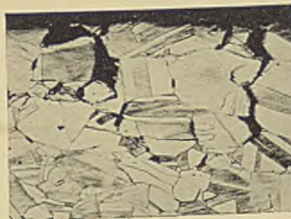
FIG. 1: The intercrystalline crack shown here is the result of a sharp blow while the metal is at black heat. These conditions may occur in handling metal after annealing. Transverse edge section Mag. 75X.
