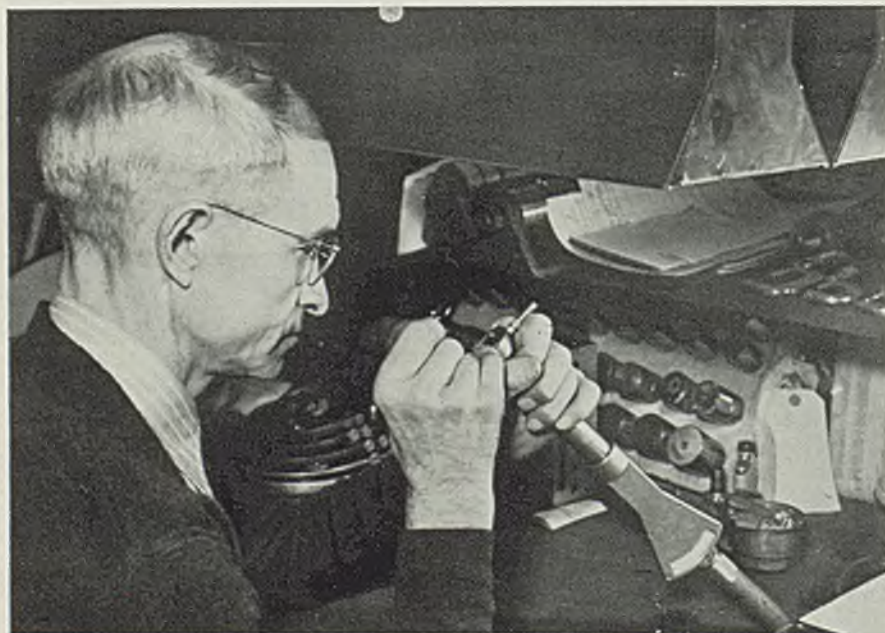
■ For peering into differentials Pontiac has adopted this Swedish internal gage to check bearing diameters in the differential carrier. It replaces the common "plug" gage and was adopted because it not only measures but records the measurement on the handle dial, thus making a selective fit possible. Differential bearing diameters are kept within one-thousandth of an inch. Here Van Smith, veteran Pontiac gage expert, makes a periodic check of the new gage's accuracy
