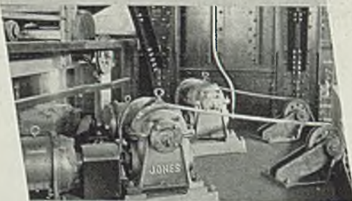
Two of a battery of 10 Jones Worm Gear Door Hoists for operating open hearth furnace doors.
