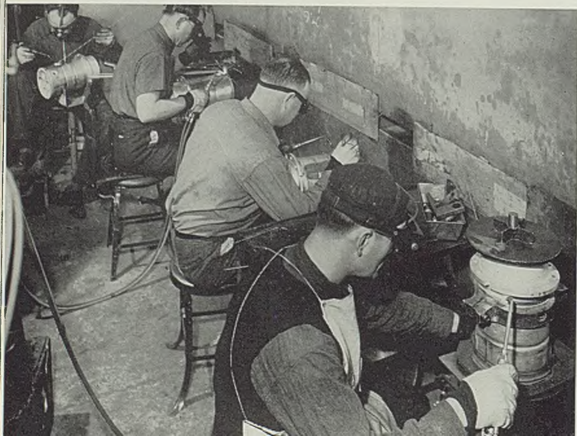
Fig. 6—Gas welding stainless steel water jacket to cylinder barrel. Operators in background are making top, side and outlet fitting welds, using 18-8 chrome-nickel rods, with columbium. Operator in foreground is making bottom weld, using no welding rod. Cylinder is filled with oil and sealed. This oil, together with a heavy copper clamp placed just below the weld line, insures rapid conduction of heat away from the area of the weld. Fixture is rotated slowly as weld progresses
