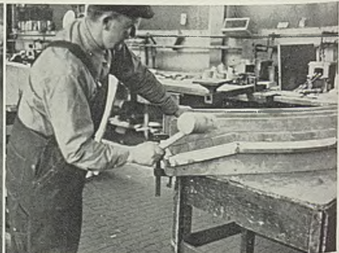
Fig. 4—Forming in three dimensions cannot be handled on the bending brake so wooden forms are used for certain parts as shown here at right below
