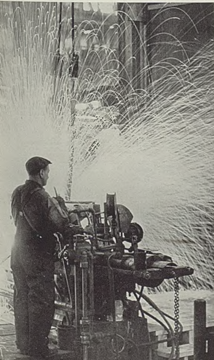
■ Not a Fourth of July display, but one which may well tie in with the national defense program. The huge fan of flying sparks is caused by flash welding, as two semi-circular pieces of steel are fused into a magnet-frame for a direct current electric motor. Asbestos curtains hanging from 30 feet above the floor restrict the sideward flight of the sparks shooting from the welder. Photo, General Electric Co.
