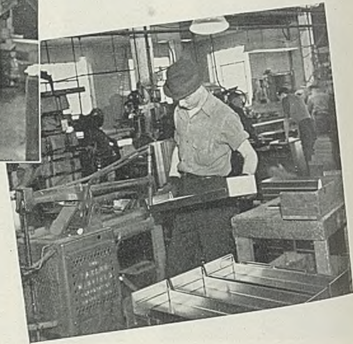
Fig. 1—This is start of the drawer production line—a series of punch press and welding operations. Fig. 2—End of drawer production line shown below—assembling backs of drawers in place by spot welding
