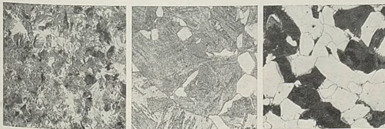
Fig. 2—Typical microstructures. Left, mixed structure of steel 4 given heat treatment EE (see Table II). Fig. 3—Grains containing acicular structure, developed in steel 2, given heat treatment H. Fig. 4. (Right)—Grains of ferrite and pearlite in steel 2, given heat treatment G. All are shown at 100 diameters
