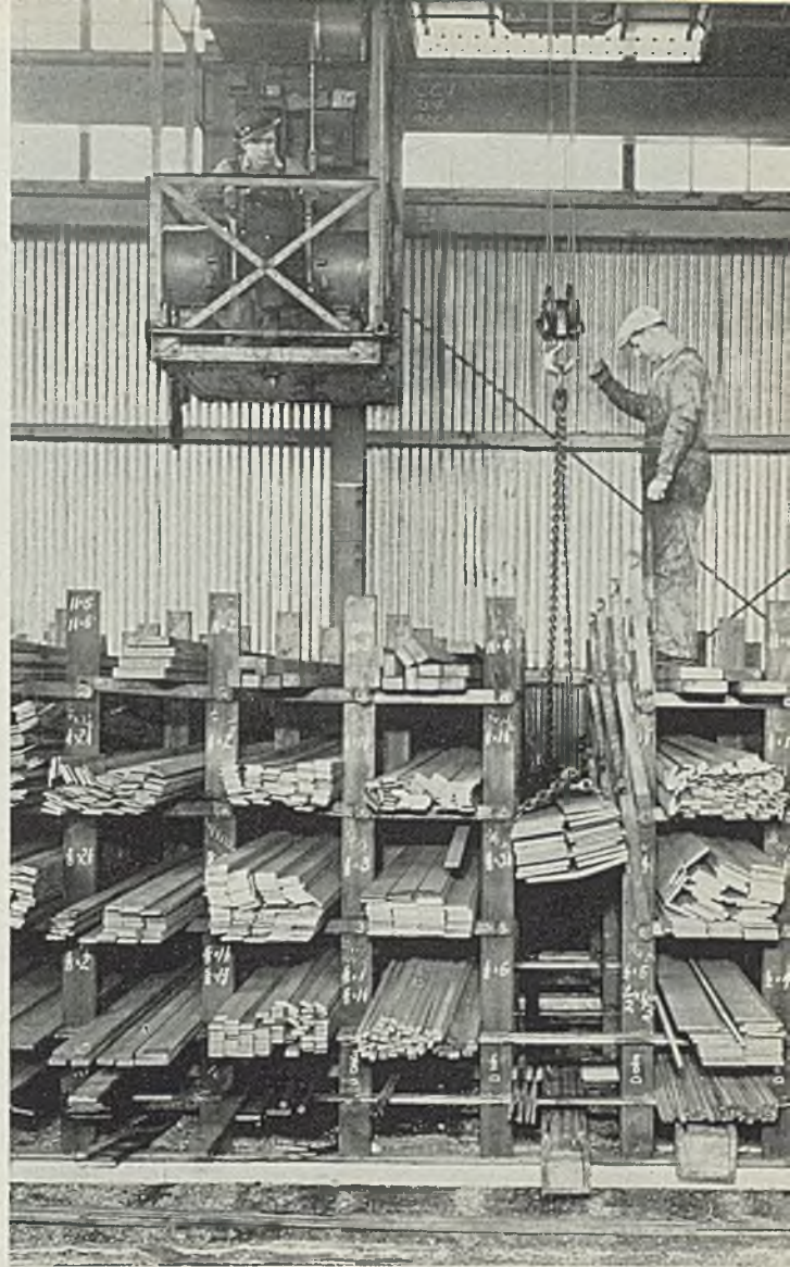
Fig. 1—This shows how cross bars are hinged to permit removal of steel from lower sections—a novel arrangement facilitating access to all the steel
