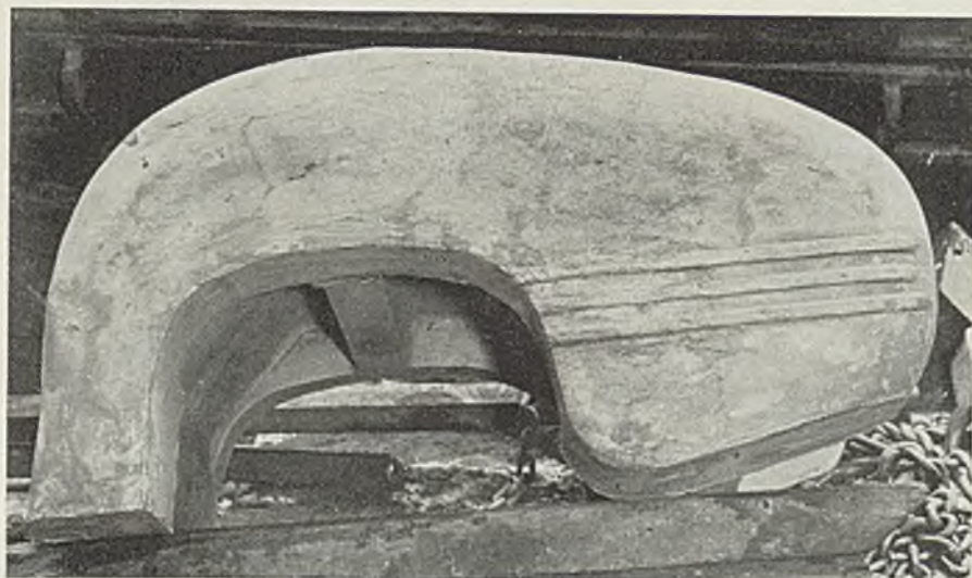
■ Rear fender punch casting weighing 6500 pounds for one of the leading models. Made of high-tensile, chrome-molybdenum iron, the punch is flame hardened along the three speedlines to prevent undue wear
