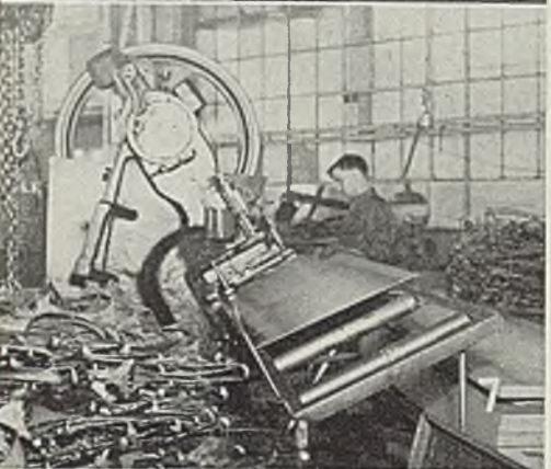
Fig. 8—Here two roller conveyors carry finished parts from stock room to assembly conveyors
