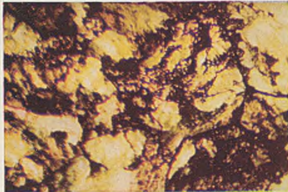
E Pearlitic Grain Size in High Carbon patented rod. Ordinary light (left). Plane polarized light taken on Kodachrome film (right). Magnification 200X—Enlargement 2X.
