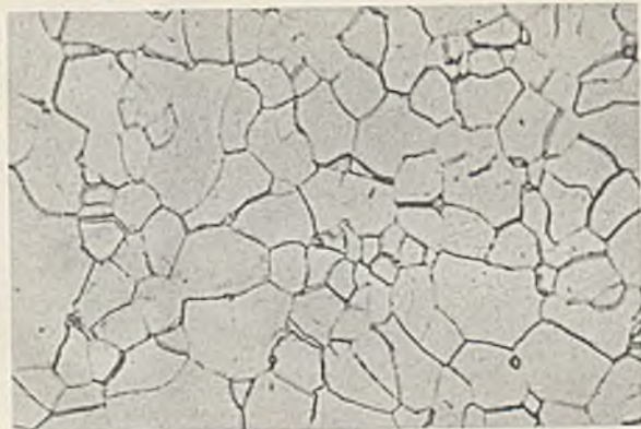
A Comparison between ordinary light (left) and Sensitive Tint Illumination taken on Kodachrome film (right) on ferrite in low carbon annealed steel wire. Magnification 200X—Enlargement 2X.
