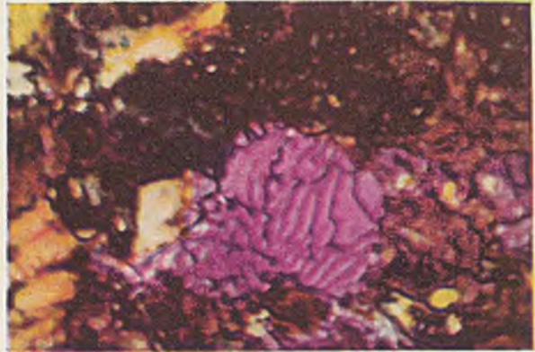
D Coarse Pearlite in high carbon patented wire. Ordinary light (left). Sensitive Tint Illumination taken on Kodachrome film (right). Magnification 1000X — Enlargement 2X.
