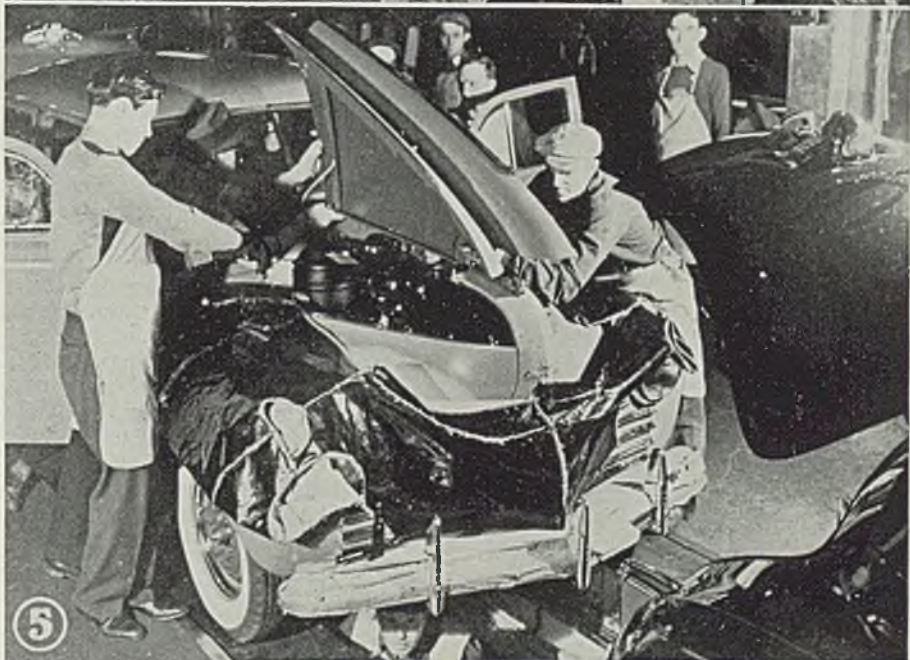
Fig. 4—At 10:39 the body is dropped into place by a traveling crane. The body is firmly bolted into place and toeboards, draft pads and clutch, brake and accelerator pedal pads are put on the car. Front and rear bumpers, batteries and all the wiring between the body and the chassis are installed and a score of other operations take place. Men in pits beneath the conveyor assemble parts to the underside of the car
