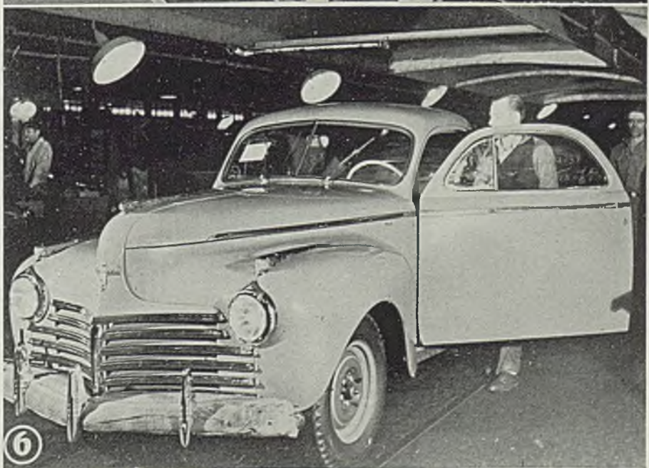
Fig. 5—At 10:51 the hood is installed. Water, alcohol and anti-rust compound are placed in the radiator and gasoline in the fuel tank. An automatic device lines up the front wheels so the steering wheel may be placed properly
