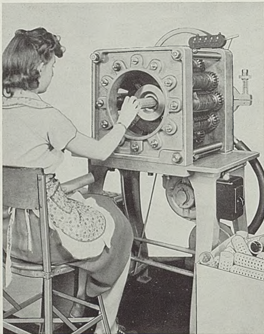
Fig. 2—Machine setup to punch by the method described. Note the 12 eccentric shafts evenly spaced around the object and carrying the punches. Note operator cannot get fingers under punches
