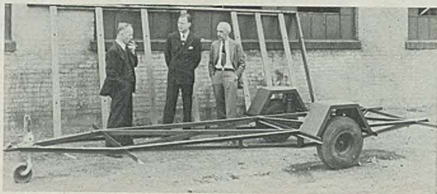
All-steel trailer chassis with independently sprung wheels, eliminating rear axle
