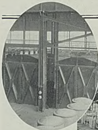
LEFT— Rust of Pittsburgh built a battery of these box annealing furnaces for the Wheeling Steel Corp., and insulated them throughout with Armstrong's N-16 Insulating Brick for accurate temperature control and operating economy.
