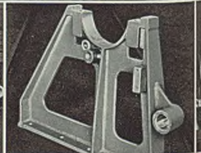
5. Another view of side frame machinery supports. Also made from plates and rounds.
