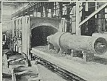
SWINDELL-DRESSLER report fuel savings of 65% with this gas-fired, car-type annealing furnace which they built for a Pittsburgh manufacturer. Insulation is 9" Armstrong's EF-22 Insulating Fire Brick backed up with 9" Armstrong's N-16 Insulating Brick.
