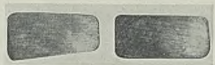
Enlarged cross-section of the wire used in the construction, shown at left, and right, the shape assumed by the wire as it is coiled
