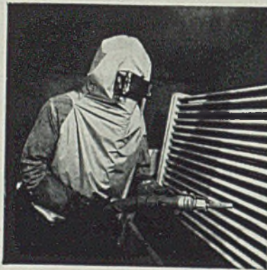
Abrasive mask developed by Mine Safety Appliances Co. for use in shot and sand blasting work
