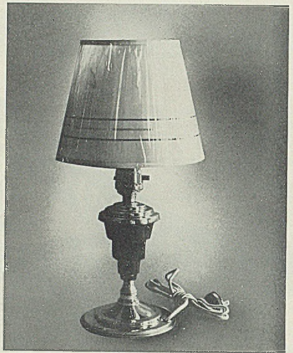
Fig. 1—Three spun metal sections make up the body of this novelty lamp
