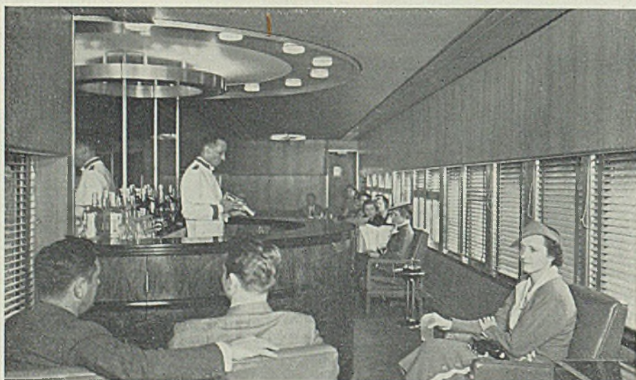
Semicircular bar in lounge is backed by mirrors to create illusion of width and spaciousness. Brilliant lighting provided directly from lens bulbs is enhanced by indirect lighting from bulbs in suspended aluminum trough. Ceiling plates and trough are of scratch brushed aluminum, with paper finish on ceiling
