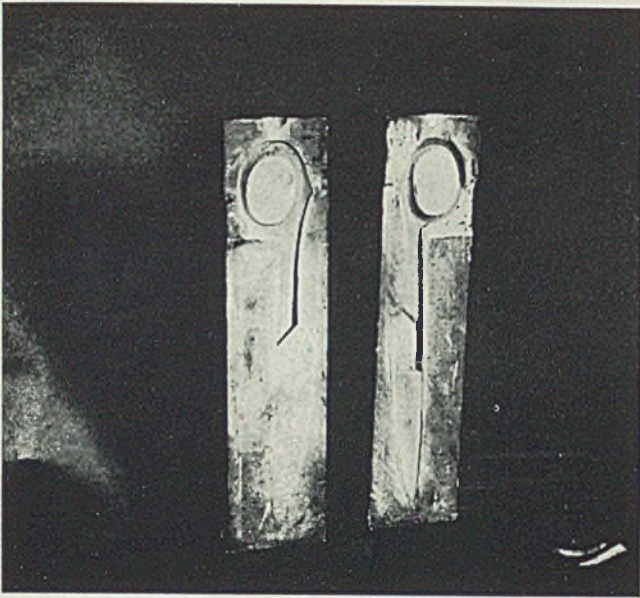
Fig. 4—From the hobs plaster of paris molds are made, in which lead castings are poured to show the exact size of the finished product
