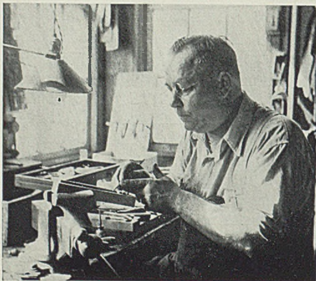
Fig. 3 — Expert die-sinkers finish the hobs which must have perfectly smooth surfaces
