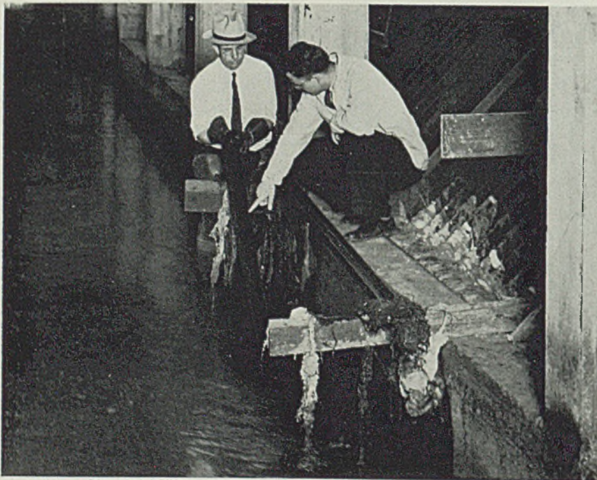
Test panels were inspected at regular intervals by paint technologists. The panel undergoing inspection was exposed to incoming raw sewage
