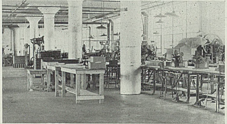
FIG. 5—Many of the operations incidental to camera production are performed in a department equipped with small presses. Even in this department, corrugated steel box skids provide a convenient means for handling parts
