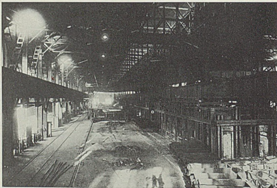
Fig. 9—General view of basic open hearth shop equipped with eight 110-ton furnaces. The No. 2 furnace is being charged. At right front are shown charging cars with scrap pans
